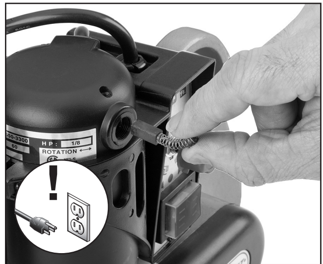
Figure 21. Brush set replacement.
